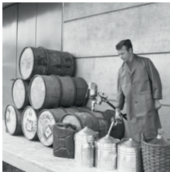
Manual filling with drum pump and FM cylindrical piston meter in 1960.
