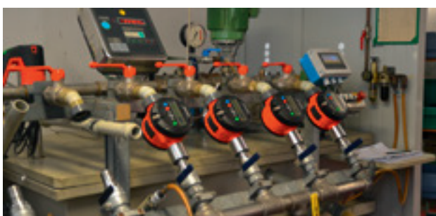
Each flow meter is checked and calibrated - 100 % quality control!
